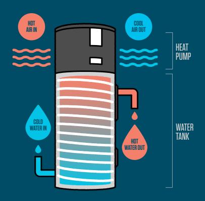
Heat pump water heaters use surrounding heat and transfer it to the water in your tank, making it **2x as efficient** as an electric water heater. Our warm climate year-round makes Hawai'i an ideal place for this energy-saving measure.
