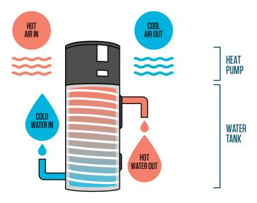
This incredibly smart technology pulls in warm ambient air from outside of the tank to heat water and transfers cool air out. It is typically installed in a garage or closet – nothing on your roof. At nearly **twice the efficiency** as a conventional water heater, you **pay up to 40% less for energy!** You may even experience a cooling effect in the space where you keep your tank due to the air transfer.
